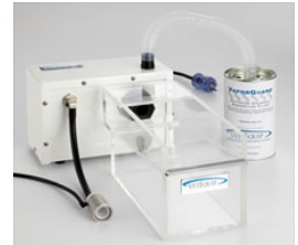
Examples of active scavenge engineering controls from left to right; fume hood and active scavenging cube
